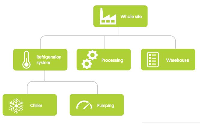
Figure 14: Potential sub-metering installation points
