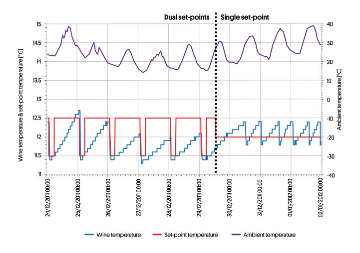
Figure 36: Dual Setpoint Load Shifting
